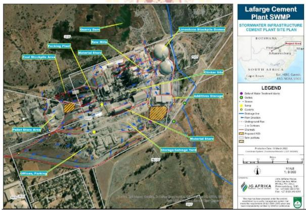
Figure 4: Lafarge Lichtenburg Cement Plant Proposed Stormwater Management Infrastructure
